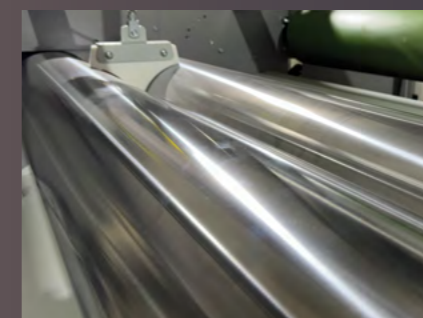
Hard Chromium-Coated Adhesive Transfer Cylinders
