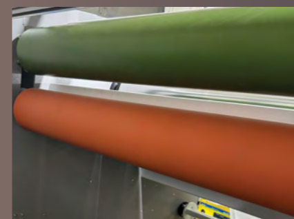
Teflon & Silicon-Coated Squeezing Rollers
